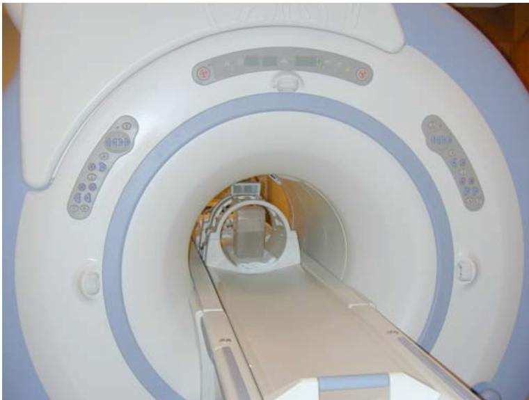
**Fluid-filled phantom with the markers inside of the head RF coil in the 3-Tesla MR system.**
