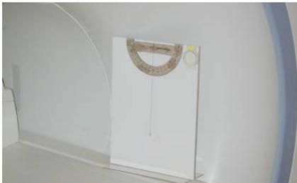
**FIGURE 4. Example showing position for the fluoroptic thermometry probe relative to the marker used to record temperatures during the MRI-related heating experiments performed at 3-Tesla.**
